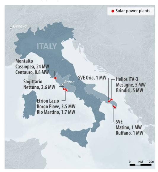
All the PV Plants are equipped with modules (e.g. Yingli Solar YL230P-29b, Sunpower SPR-305-WHT, Trina Solar TSM-225PC05) and inverters (e.g. Siemens SINVERT 1000 MS TL, Bonfiglioli RPS 450 TL 170TL, SMA SC630HE) and are managed by O&M operators.
